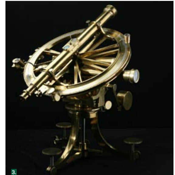
1. Armillary sphere, 1560-1580, unsigned; 2. Gunner's level, early 17th century, Heinrich Stolle, Prague; 3. Astronomical theodolite, 1816-1818, Reichenbach, Utschneider and Liebherr, Munich
