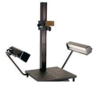
copy stand with adjustable camera and lamp positions
